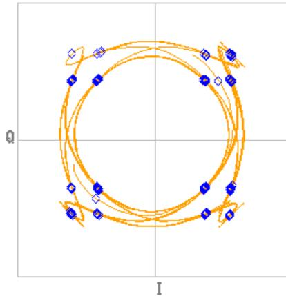
Figure 2: OpenBTS default configuration, phase error  $4.98^\circ$  RMS,  $14.95^\circ$  peak
