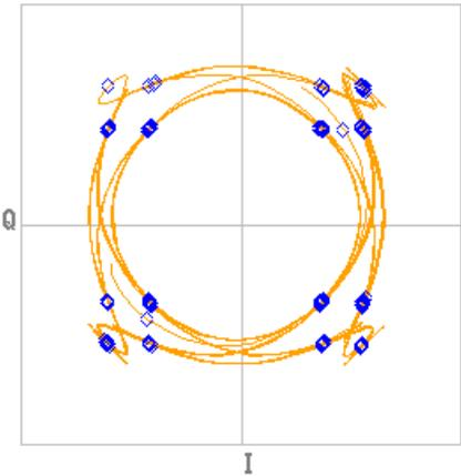
Figure 12: OpenBTS-USRP1 phase error, 1 sample per symbol, C0 pulse, 4.98° RMS, 14.95° peak
