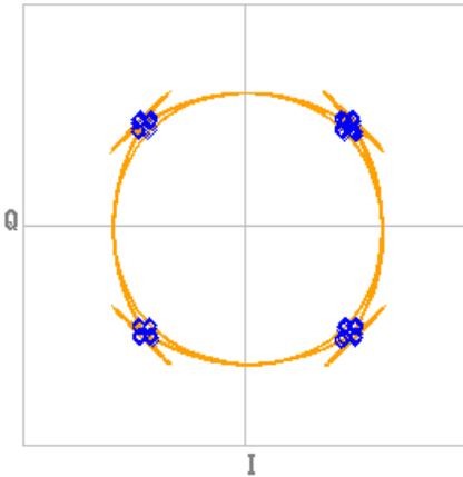
Figure 13: OpenBTS-USRP1 phase error, 4 samples per symbol, C0 pulse, 1.92° RMS, 5.44° peak
