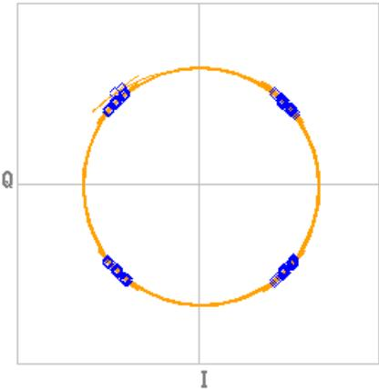
Figure 14: OpenBTS-USRP1 phase error, 4 samples per symbol, C0 and C1 pulses, 1.66° RMS, 4.53° peak
