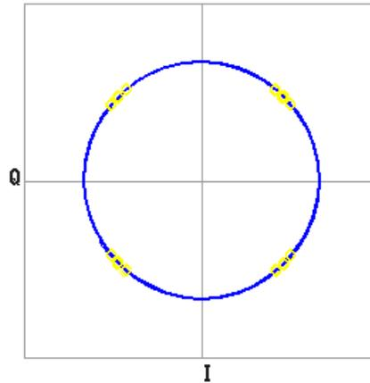
Figure 1: GSM reference signal, phase error  $0.29^\circ$  RMS,  $0.85^\circ$  peak
