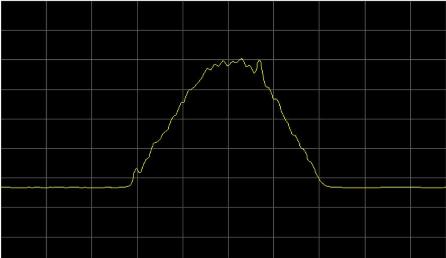
Figure 4: Undersampled OpenBTS spectrum with 1 samples-per-symbol, 1 MHz span
