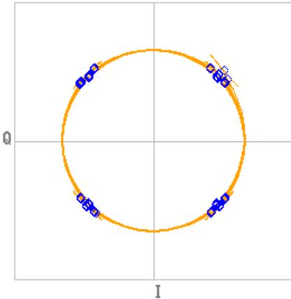
Figure 15: OpenBTS-USRP2 phase error, 4 samples per symbol, C0 and C1 pulses, 1.14° RMS, 2.97° peak
