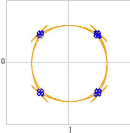
Figure 5: OpenBTS signal, 4 samples per symbol, phase error 1.97° RMS, 5.08° peak
