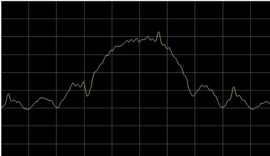
Figure 3: Oversampled OpenBTS spectrum with 8 samples-per-symbol, 1 MHz span
