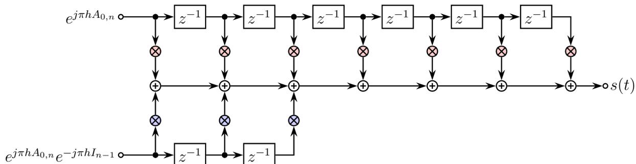
Figure 11: Combined tapped delay line for linearized GMSK pulses C0 and C1
